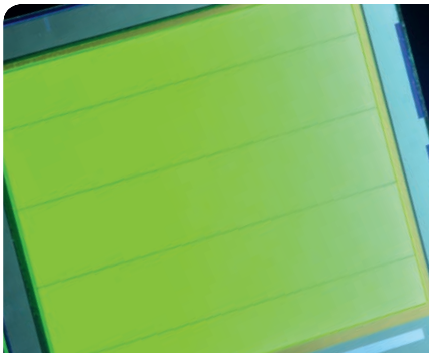
Homogenous luminosity for OLEDs thanks to micro-scale conductor paths. © Philips
